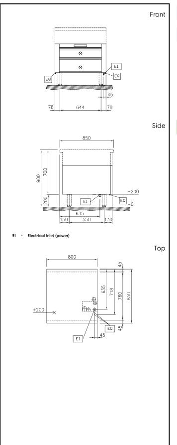
Electric Supply voltage: 230 V/1N ph/50 Hz Key Information: External dimensions, Width: 800 mm External dimensions, Depth: 850 mm External dimensions, Height: 450 mm **Cupboard Cavity Dimensions** (width): 650 mm **Cupboard Cavity Dimensions** 325 mm (height): **Cupboard Cavity Dimensions** (depth): 530 mm Cabinet temperature range: 30-120 °C Net weight: 44 kg
